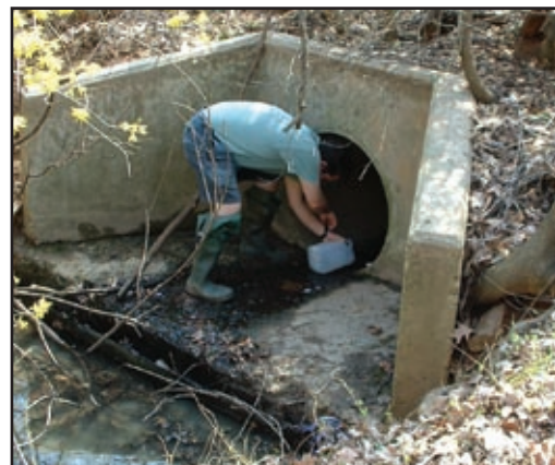
Figure 30: Measuring flow (as volume per time)
